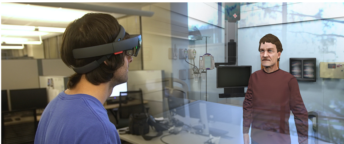
Figure 3. Augmented Reality technology can overlay synthetic objects onto a real-world environment. This mockup represents the possibility for projecting a virtual patient in a hospital room using a device such as the Microsoft HoloLens.
