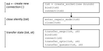
Figure 4: Procedure for TCP connection relocation
