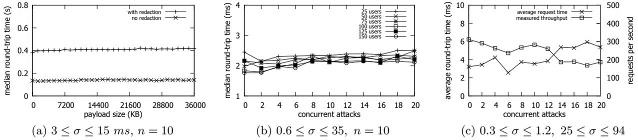
**Figure 6: Performance benchmarks.** (a) Effect of payload size on malicious HTTP request round-trip time. (b) Effect of concurrent attacks on legitimate HTTP request round-trip time on a single-node VM. (c) Stress test illustrating request throughput for a 3-node, load-balanced RedHerring setup (workload  $\approx 5K$  requests).
