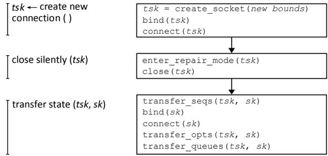
Figure 4: Procedure for TCP connection relocation
