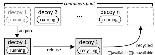
Figure 2: Linux containers pool and decoys life cycle
