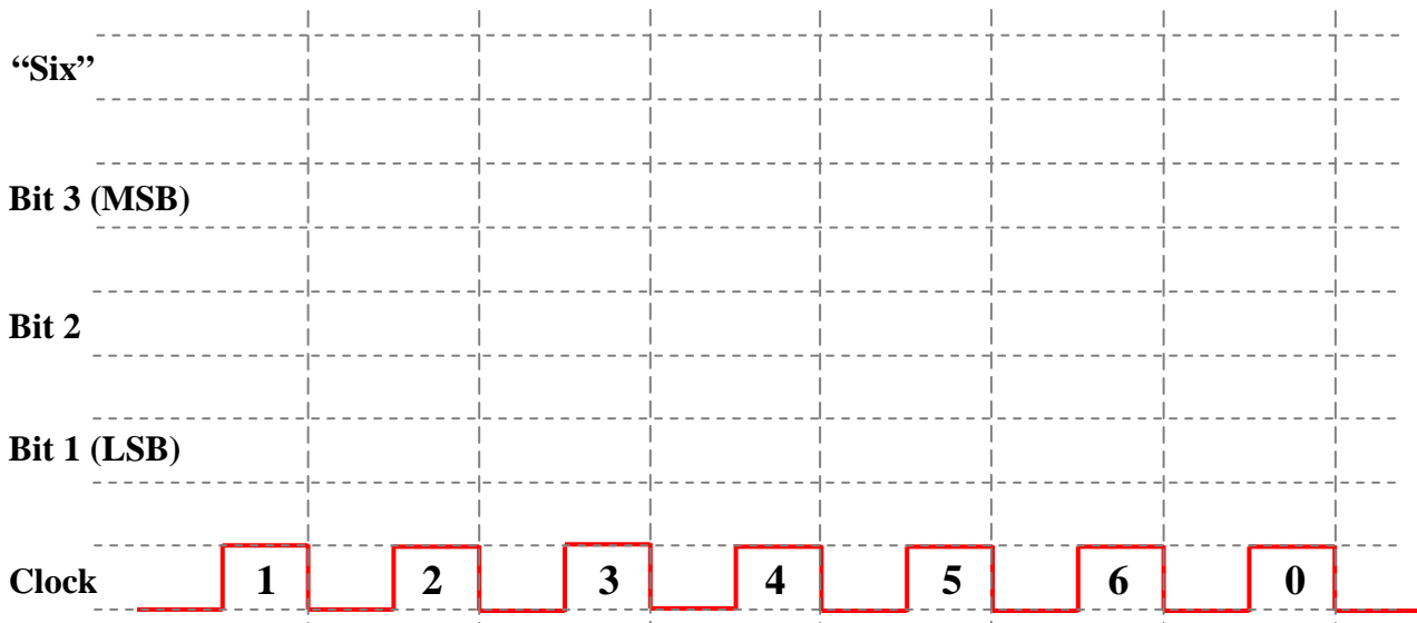
Timing of Modulo-7 Counter
