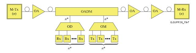
Figure 8-7 – Example of a bus structure with optical amplifiers and one OADM
