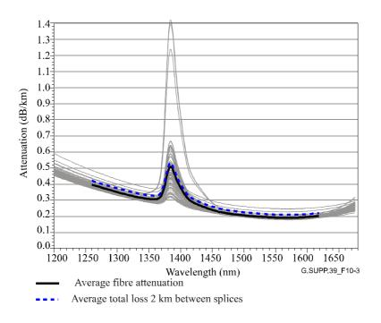
Figure 10-3 – Measured fibre attenuation and splice loss in installed G.652 A&B cable – Cables installed around 2000
