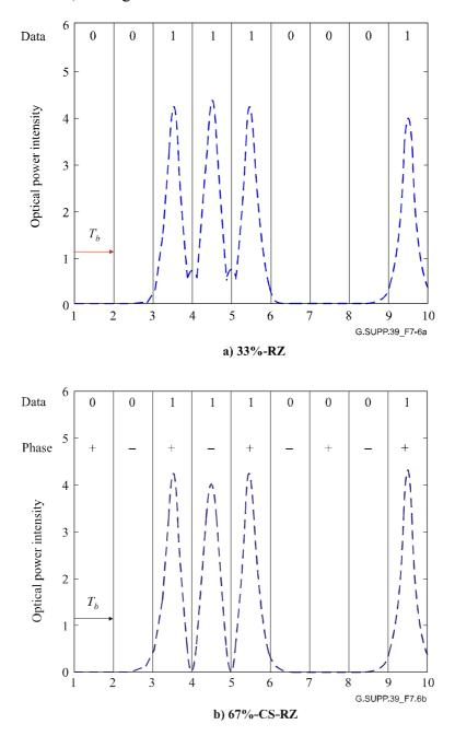
Figure 7-6 – 40-Gbit/s pulse form after accumulated dispersion of 20 ps/nm
