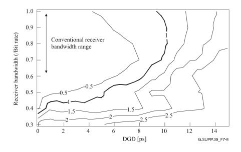
Figure 7-8 – Contour map for DGD tolerance (RZ-50%)
