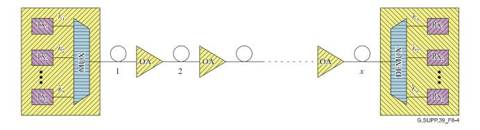
Figure 8-4 – Example of a WDM point-to-point link
