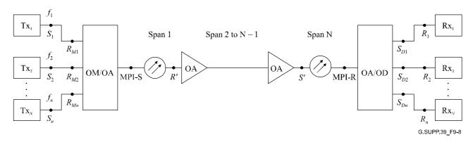
Figure 9-8 – Representation of optical line system interfaces (a multichannel N-span system)
