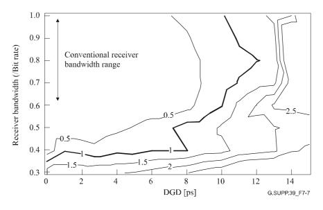
Figure 7-7 – Contour map for DGD tolerance (RZ-33%)
