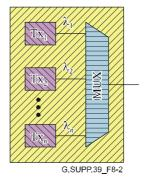
Figure 8-2 – Example of a multichannel transmitter realization scheme
