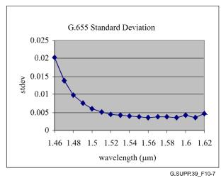
Figure 10-7 – Average and standard deviation of difference in attenuation coefficient from 1550 nm – G.655
