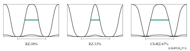
NOTE – The thin bar indicates the bit period T and the thick bar indicates the pulse width, corresponding to duty cycle.
