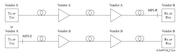
Figure 12-4 – Multi-span single interface transverse compatibility
