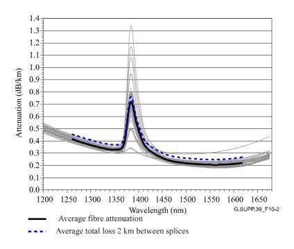
Figure 10-2 – Measured fibre attenuation and splice loss in installed G.652 A&B cable – Cables installed before 1990
