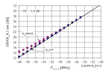
Figure 9-12 – OSNR versus received optical power measurement: with noise correction (n cor) and without noise correction (n uncor) at the signal channel wavelength
