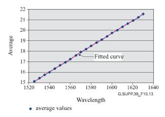
Figure 10-13 – Average chromatic dispersion coefficient of G.652 fibre
