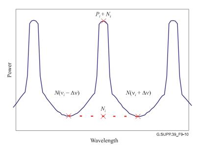
Figure 9-10 – Inaccurate OSNR measurement due to noise shaping
