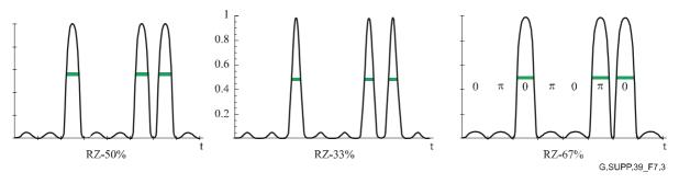
NOTE – The bar indicates FWHM and the duty cycle of the pulses.  $\pi$  and 0 indicate the phase change of RZ pulses at CS-RZ-67%.
