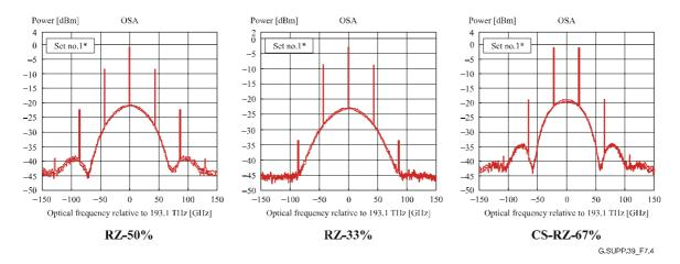
Figure 7-4 – Optical spectra of RZ formats
