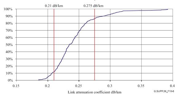
Figure 10-8 – Probability of loss being met vs link 1550 nm attenuation coefficient for links > 20 km
