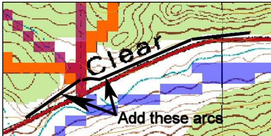
Figure 2-8: Roadway collection stream arcs
